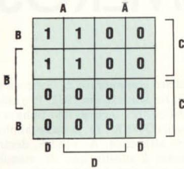
$$\begin{aligned} & ABC\bar{D} + ABCD + A\bar{B}C\bar{D} + A\bar{B}CD = \\ & = ABC(\bar{D} + D) + A\bar{B}C(\bar{D} + D) \\ & = ABC + A\bar{B}C \\ & = AC(B + \bar{B}) \\ & = AC \end{aligned}$$
