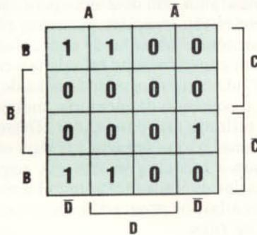
$$\begin{aligned} & ABC\bar{D} + ABCD + \bar{A}BC\bar{D} + \bar{A}BCD + A\bar{B}C\bar{D} \\ & = ABC(\bar{D} + D) + \bar{A}BC(\bar{D} + D) + A\bar{B}C\bar{D} \\ & = ABC + \bar{A}BCD + A\bar{B}C\bar{D} \\ & = AB(C + \bar{C}) + \bar{A}BCD \\ & = AB + \bar{A}BCD \end{aligned}$$
